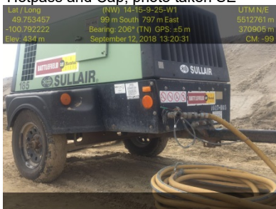
Sept 12/18 Description & Location: SSKP 822+300 Not a self contained unit for spills Needs spill tray Environmental Coordinator said they need them
